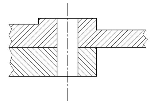
B) The bottom plate is drilled to the depth of 30 mm before being tapped to the depth of 25 mm for an M16 Hexagon Socket Head Cap Screw. The capscrew is 30 mm long and has a thread length of 20 mm. Draw the screw in assembly.
